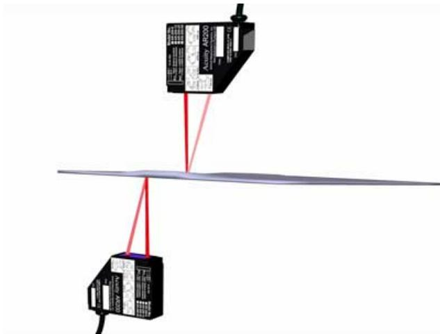
For precision thickness applications, it is imperative that the sensors are aimed directly opposite to each other. For in-process thickness measurements, an alignment offset could mean the difference between satisfactory and scrap product.
